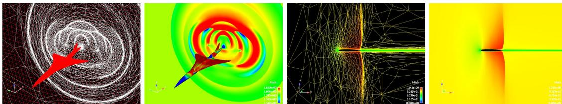
Figure 1: Adapted meshes and the associated local Mach number for the flows around the aircraft (left) and the ONERA M6 wing (right).
